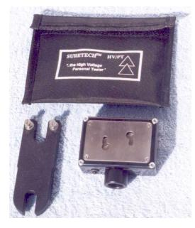
• **Battery:** A 9 volt Alkaline PP3 battery is contained in the plastic sensor box. The battery provides the source of power to operate the electronic circuits. An auto power down circuit operates after about three minutes to conserve battery power.
