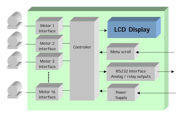
The SURETECH Motor Insulation Monitor measures insulation resistance to earth of electric motors when the motor stops. Motors running from mains 380/220Vac or 525Vac, or higher can be monitored for insulation resistance breakdown. MIM configurations are available for one motor (K125 enclosure), and also for multiple motors controlled from a motor panel.
