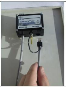
Once the CLF flasher module is mounted behind the front panel, and sensor is mounted in HV chamber, sensor cable earth is connected to earth stud, and connector clicked into flasher with RJ45 connector. RS232 cable is also clicked into flasher with supplied RJ12 connector. With different connectors no mistake can be made with wrong connectors
