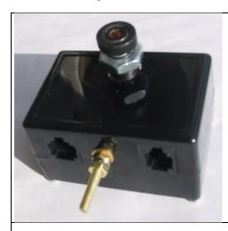
CLF flasher is mounted to the front of LV panel with one 10mm hole using a M10 bolt including locknut behind and round panel nut, with flasher LED mounted inside the M10 bolt. Earth stud is shown
